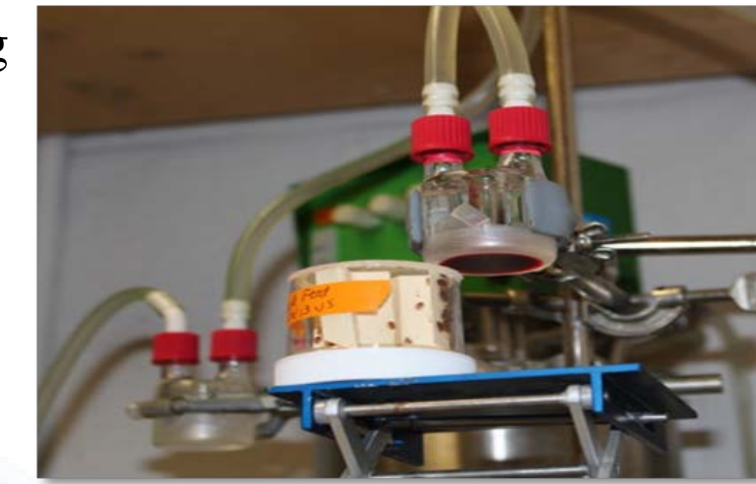
Fig 1. Artificial feeder made to simulate bed bugs feeding on a human blood meal.
